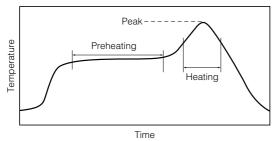
For soldering (Example: Sn/Pb)
