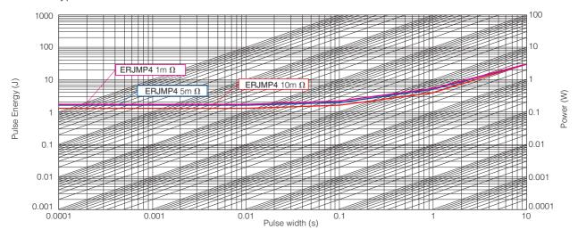
This pulse data is reference characteristic data measured under Panasonic test method and it does not guarantee the performance / characteristics of this product. (The performance / characteristics will change due to the test board, land pattern, amount and type of solder, influence of test equipment and surrounding parts, etc.) Therefore, please use it after sufficiently confirming its reliability under your using conditions.
