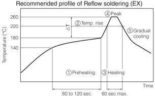
$\triangle$ T : Allowable temperature difference  $\triangle$ T  $\leq$  150 °C
