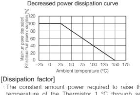
The constant amount power required to raise the temperature of the Thermistor 1 °C through self heat generation under stable temperatures.
