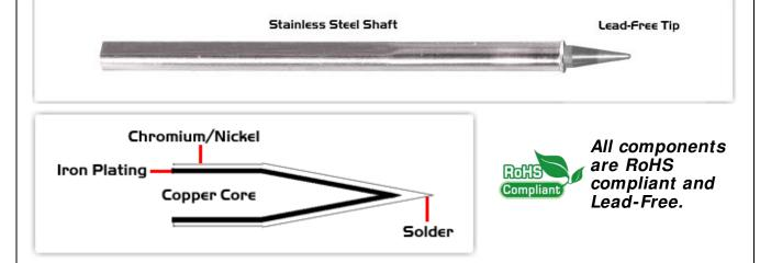
Easy Braid Co. tip cartridges will typically idle within a temperature range of +/-1.1°C. However, there is variation in idle temperature across tip geometries within an individual temperature series. Easy Braid Co. offers a wide variety of tip geometries from 0.25mm fine point tip to 5mm chisel. The length and geometry of a tip will have an influence on the tip idle temperature. To accurately measure idle temperature it will depend greatly on the measurement method,
