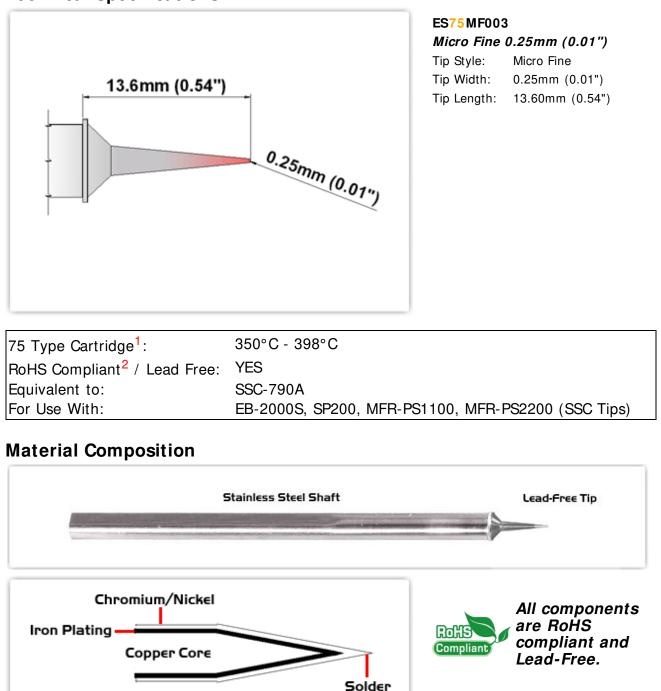
Easy Braid Co. tip cartridges will typically idle within a temperature range of +/-1.1°C. However, there is variation in idle temperature across tip geometries within an individual temperature series. Easy Braid Co. offers a wide variety of tip geometries from 0.25mm fine point tip to 5mm chisel. The length and geometry of a tip will have an influence on the tip idle temperature. To accurately measure idle temperature it will depend greatly on the measurement method,
