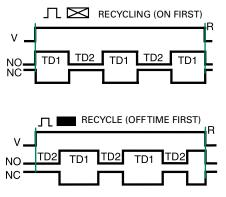
V = VoltageNO = Normally Open Contact NC = Normally Closed Contact TD1,TD2 = Time Delay R = Reset
