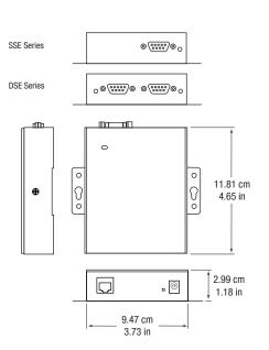
MECHANICAL DIAGRAM SSE/DSE MODELS
