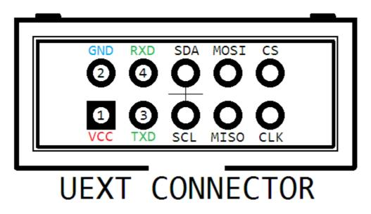
For connecting the USB<->serial cable we are interested only in pins #2, #3 and #4.
