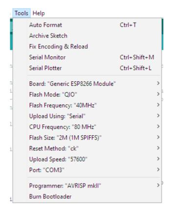
The important settings (specific for Olimex ESP8266-EVB boards) are:
