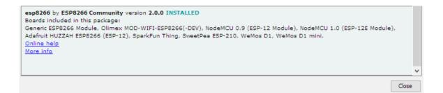
• Now at the bottom of the selector Tools → Board you should see different ESP8266 boards available. This is shown below:
