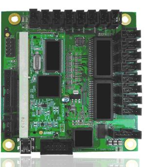
Offered with board-to-wire or board-to-board connectors
