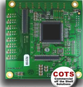
Bottom view with board-to-board connectors shown
