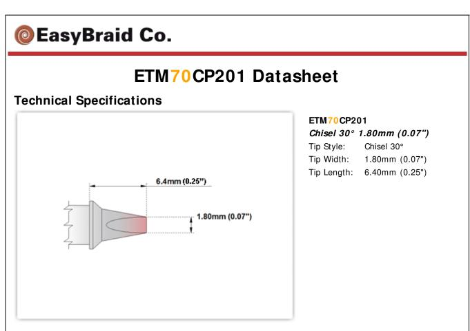
70 Type Cartridge1:350°C - 398°CRoHS Compliant2 / Lead Free:YESFor Use With:EB-5000S-1, EB-5000S-2
