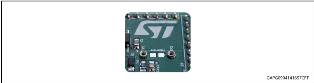
Figure 4: Mounting through-hole sense resistor
