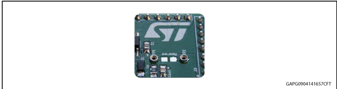
Figure 4: Mounting through-hole sense resistor
