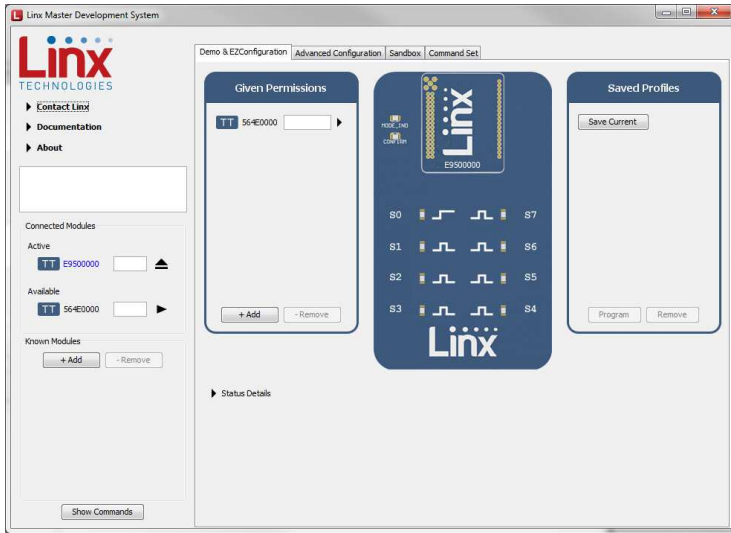
Figure 28: The Master Development System Software Demo and EZConfiguration Tab with Changes
