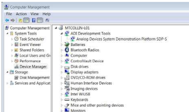
Figure 13. Device Manager: Checking that the Board Is Connected to the PC Correctly
