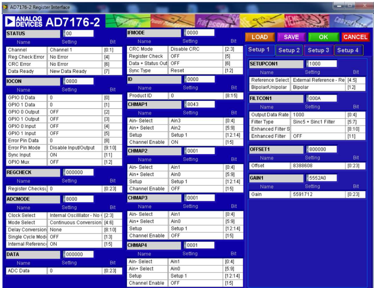
Figure 21. Configuration for Noise Test
