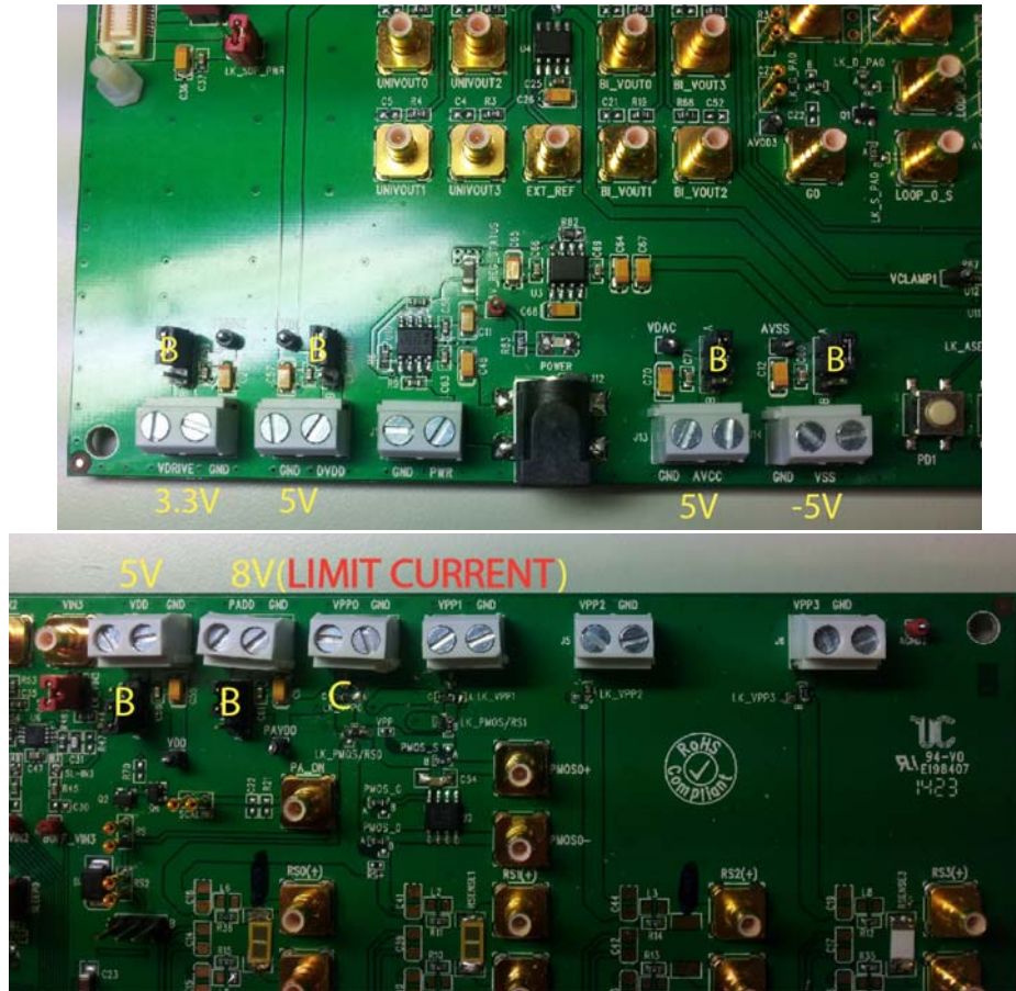
Figure 3. EVAL-AD7293SDZ Power Connections
