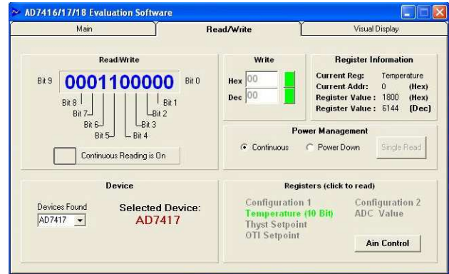
Figure 9. Read/Write Tab for AD7417 or AD7418, ADC Value Register Enabled to Read the ADC Conversion Result
