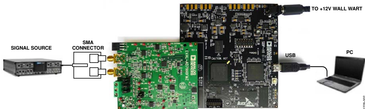
Figure 1. Setting Up the EVAL-AD7960FMCZ
