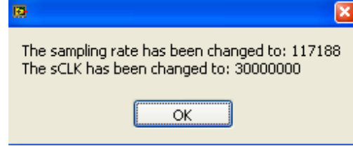
Figure 21. Software Overwritten User Settings to a Sample Rate/SCLK Rate Suitable for SDP Data Transfer
