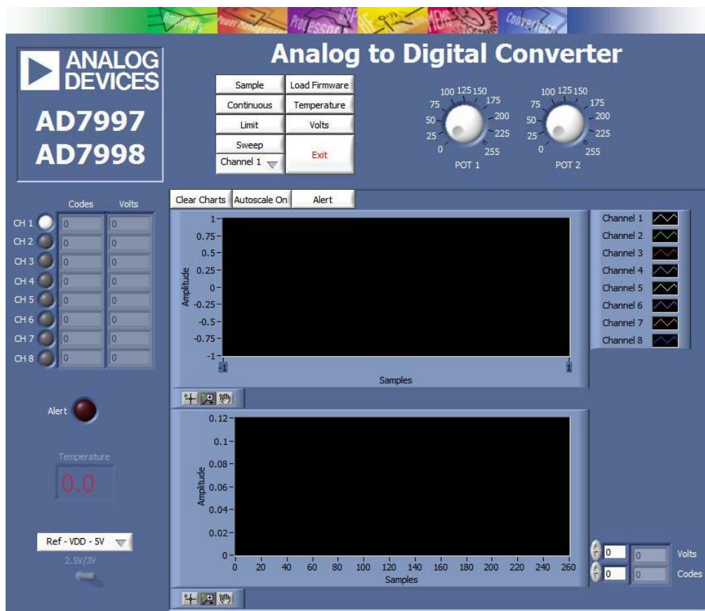
Figure 2. AD7997/AD7998 Evaluation Board Window
