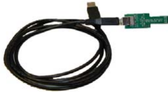
USB-TO-UART CONVERTER (ADE8052Z-DWDL1)
