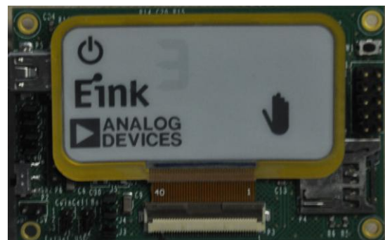
Figure 33. Display Bad Configuration for Data Logger
