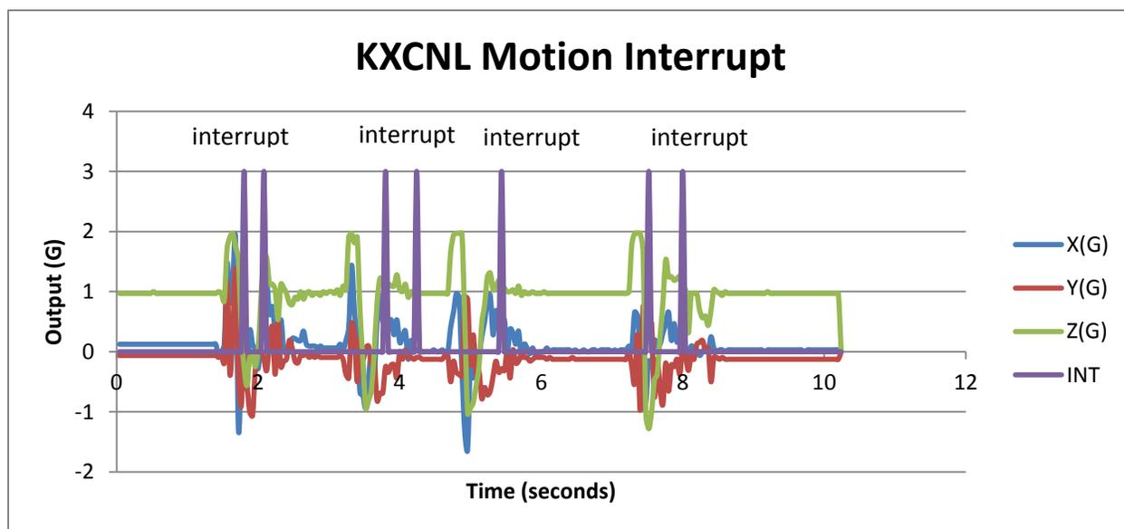
**Figure 3:** Motion Detection
