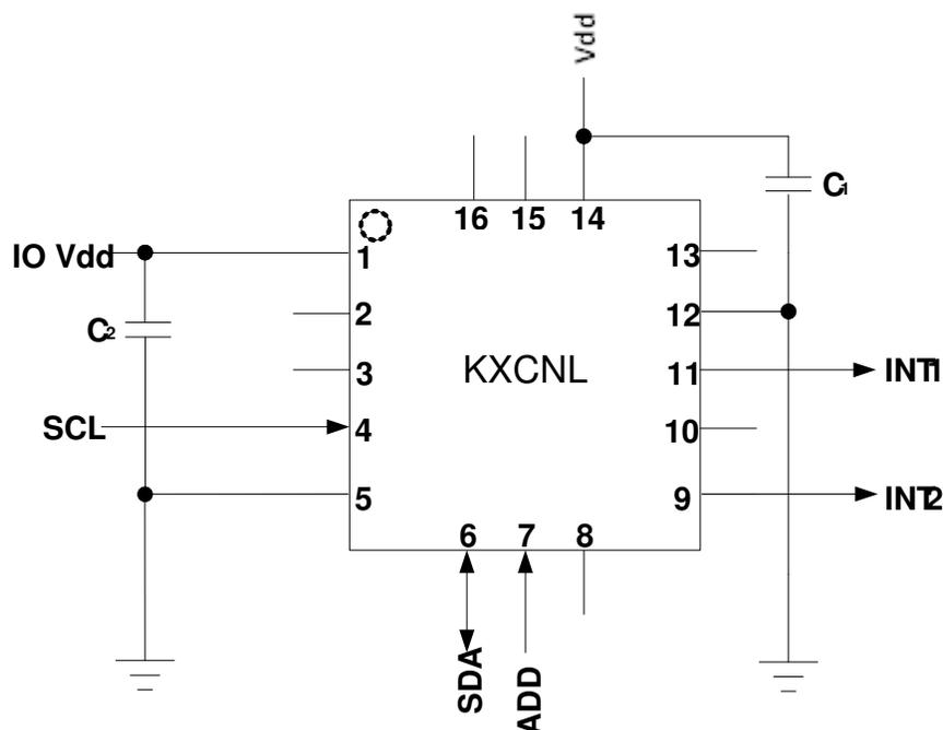
**Figure 1.** Application Schematic
