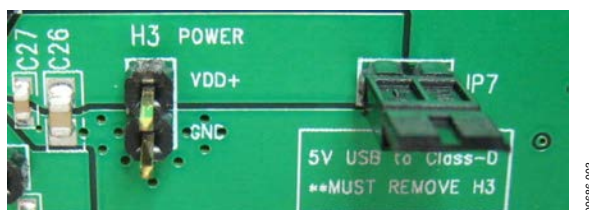
Figure 3. Connecting USB Power Supply to SSM2380
