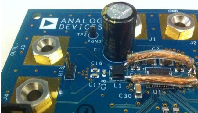
Figure 3. Board Modifications for Mono Mode
