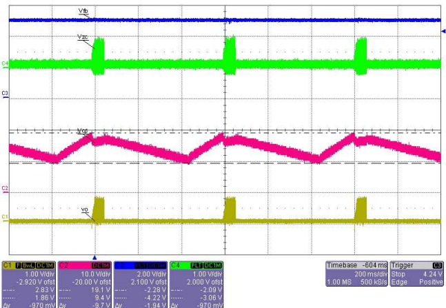
Figure 23 Output Short Circuit Protection
