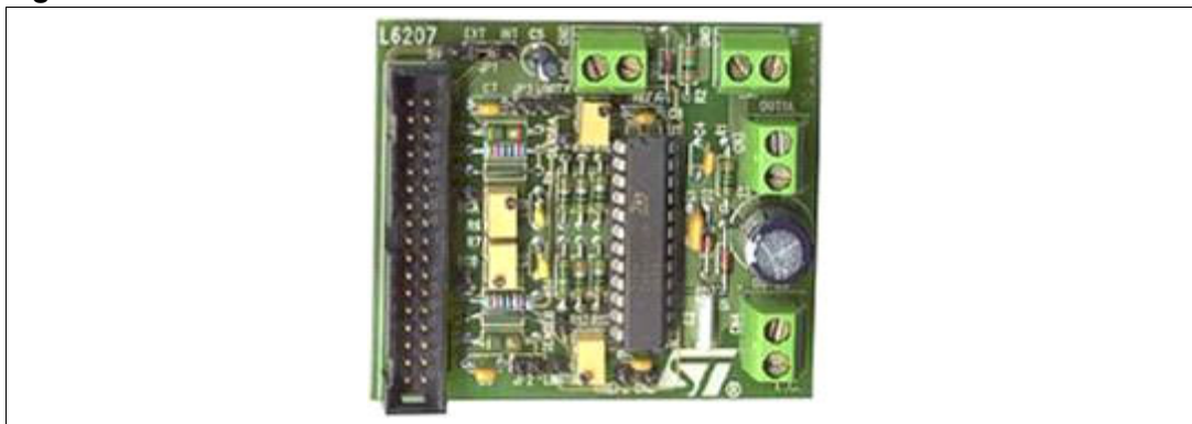
Figure 13. Motor control evaluation board EVAL6207N
