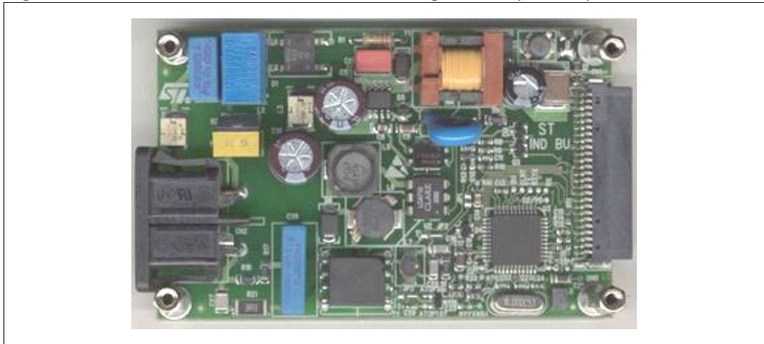
Figure 11. ST7538 dual channel reference design board (Rev 3.1)
