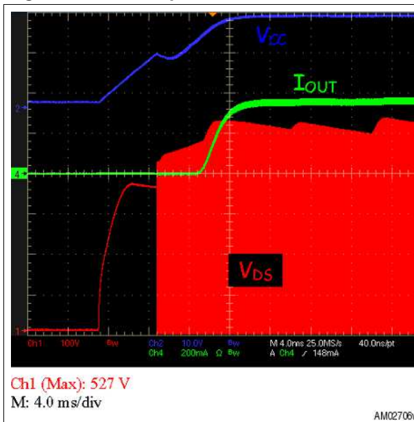
Figure 4. Start up at 230 VAC, 3 LEDs
