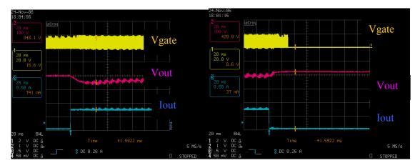
Load jump test at 85VAC, lout from 0.75A to 0A
