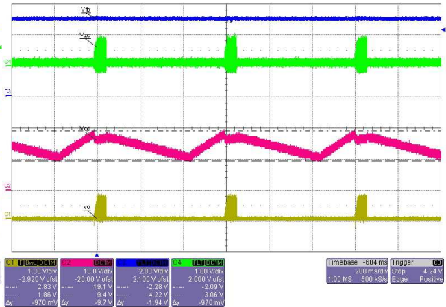
Figure 23 Output Short Circuit Protection
