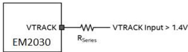
Figure 10: VTRACK Sense Circuitry (Input > 1.4V)
