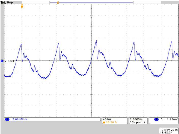
Figure 17: Output ripple V_{IN} = 5V , V_{OUT} = 3.3V
