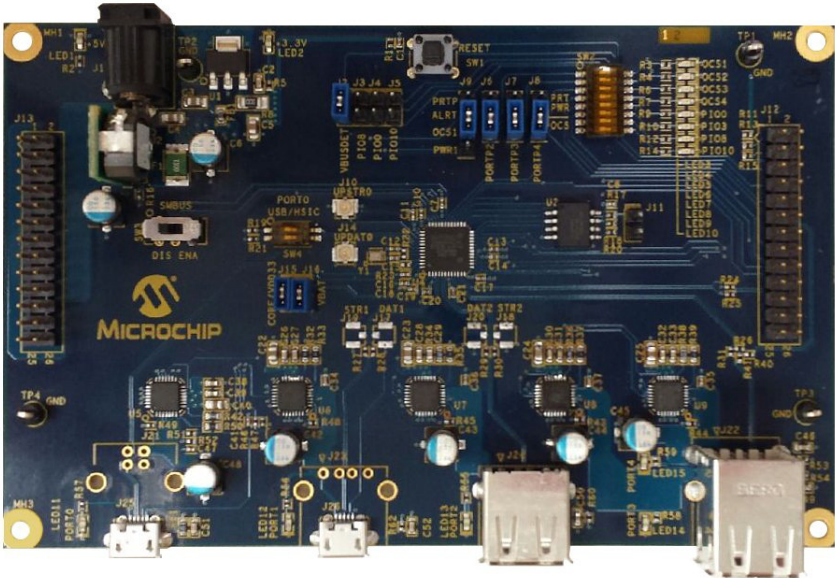
FIGURE 3-2: USB4604-1080 JUMPER CONFIGURATION
