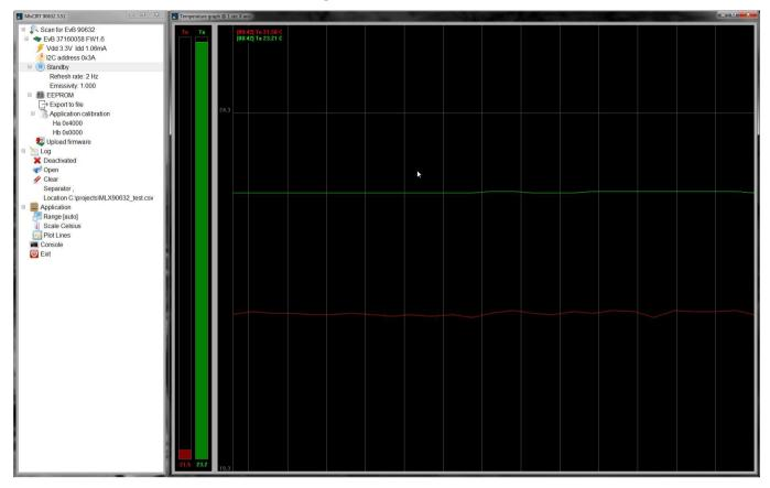
Hover the mouse pointer over the graph to show ambient and object temperature in left top corner
