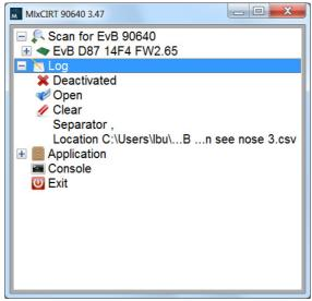
After measurement of each sub-frame, The data is stored with all measurements of one full frame (768 pixels) in one line. The next frame is stored on the next line.
