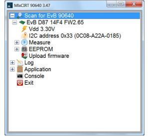
The EVB has been recognized and a sensor has been found on the PCB. The I2C address of the sensor is shown and its factory ID.
