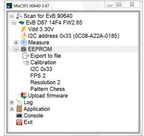
Under the EEPROM tab there is also a tab to export the EEPROM information to file and a button to upload new firmware to the EVB if needed. Here is also a tab to point the program to the file directory where a special calibration file for a specific sensor is located – if available.
