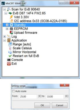
In the "Range" tab one can choose between autoscale or set the minimum and maximum temperature manually.
