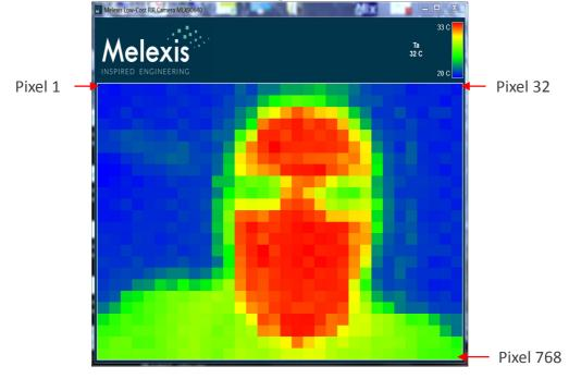
In the top right corner one can see the maximum and minimum temperature of the temperature scale, the sensor temperature Ta and the temperature To of the pixel at the pointer location. Note that the button "measure" has changed to "standby". By clicking this, one can halt the imager.
