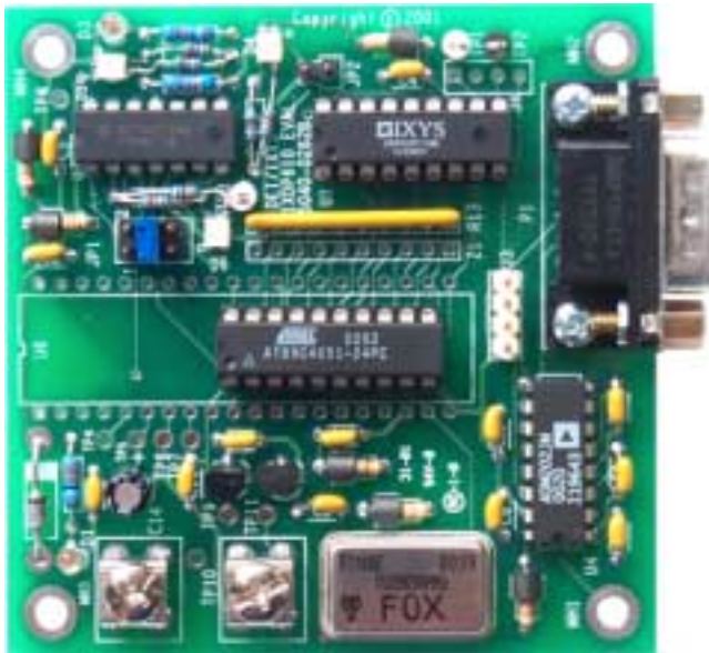
Figure 1 - EVDP610 Evaluation Board
