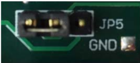
Figure 2A. (JP5: Pin 1 - 2 to Voltage Regulators)
