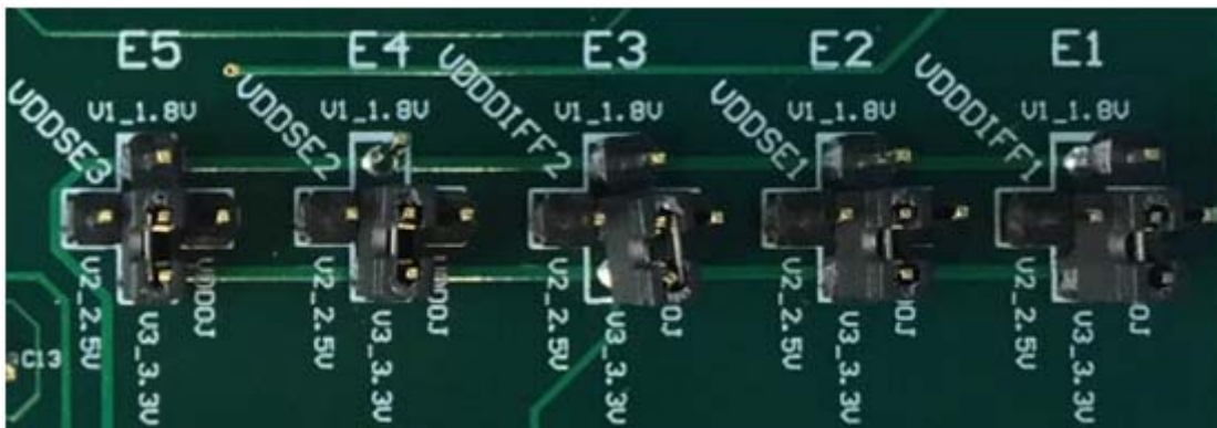
Figure 3. Jumper Configuration for On-board Voltage Regulators
