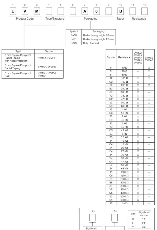
When significant number is odd, letters are assigned as shown above.
