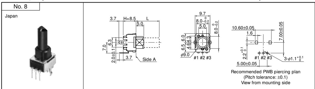
● Shaft Trims and Dimensions in mm for Type without Bushing (Drawings are at full CCW position.)
