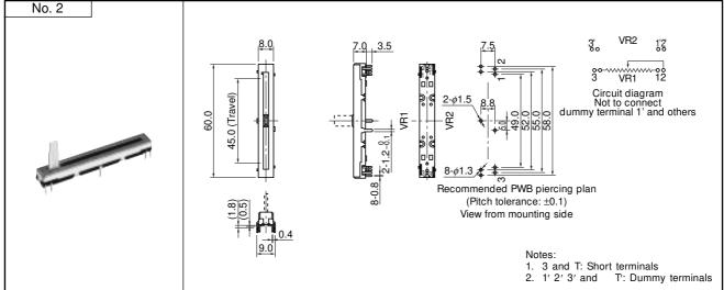
Notes: Refer to the drawing below for terminal alignment of dual slide potentiometers and single, dc version.
