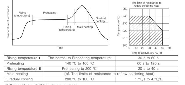
(Reflow soldering shall be within two times.)
