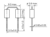
■ Taping Dimensions in mm (not to scale)
