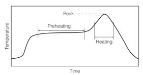
For soldering (Example : Sn/Pb)
