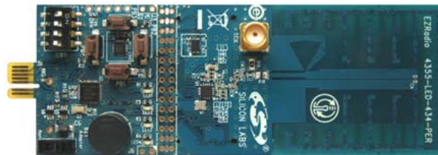
Figure 2. Si4355 RFStick 434 MHz Receiver Board (P/N 4355-LED-434-SRX)
