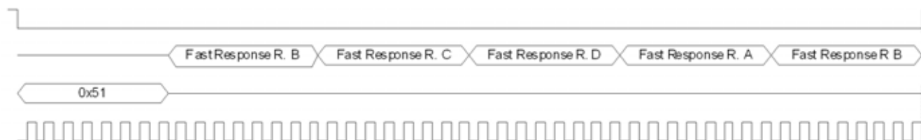
Figure 14. Reading More Fast Response Registers in a Single SPI Transaction
