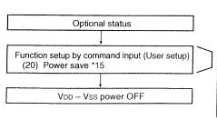
Set the time ( $t_L$ ) from power save to turning off the VDD - Vss power (VDD - Vss = 1.8 V) longer than the time ( $t_H$ ) when the potential of V5 ~ V1 becomes below the threshold voltage (approximately 1V) of the LCD panel. th is determined depending on the voltage
