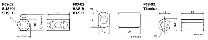
Note: 1. Dimension when mounting Electrodes.
