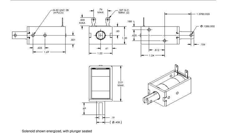
Insulation Materials: UL Construction, Class B 130°C Copper magnet wire insulation rated 155°C (class F)
