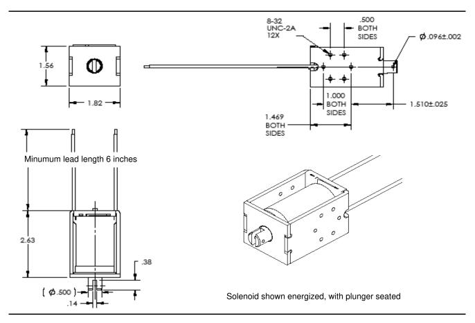
Insulation Materials: UL Construction, Class B 130°C Copper magnet wire insulation rated 155°C (class F)
